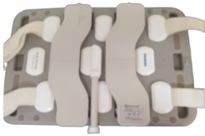
Anterior shim modules mounted on a Siemens [4] Flex body coil
